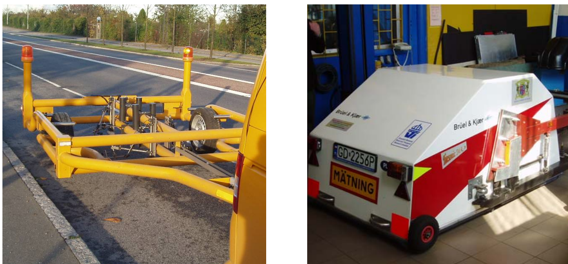
Figure 7.3: CPX noise measurement trailers can be used to monitor noise on newly laid pavements. To the left, a 'deciBella' open CPX trailer from the Danish Road Directorate/Danish Road Institute and to the right, a closed CPX trailer from the Technical University of Gdansk in Poland.
