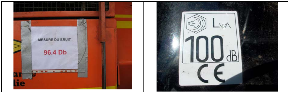
Figure 9.3: Example of noise labelling on production machinery
