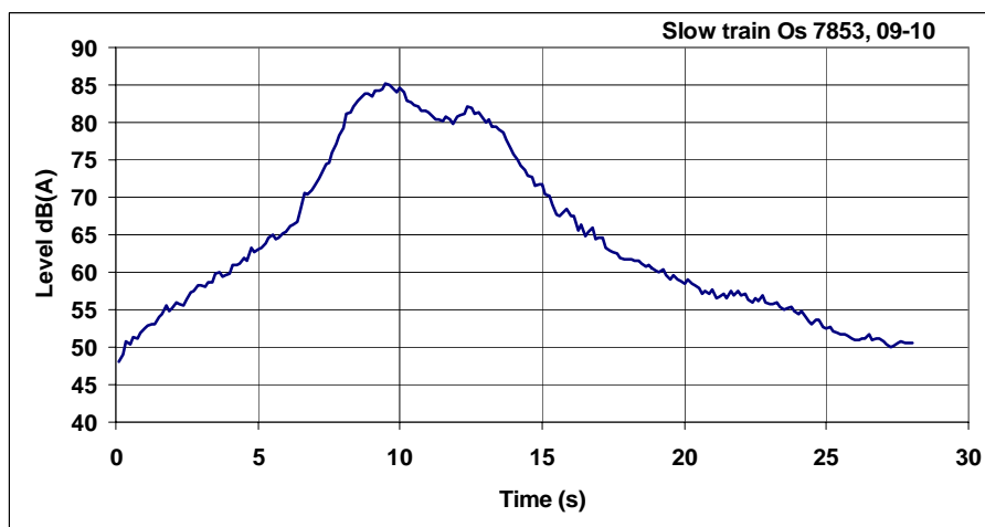
Figure 10: Measured LAF levels – Leq = 75,8 dB(A) with T = 28 s
