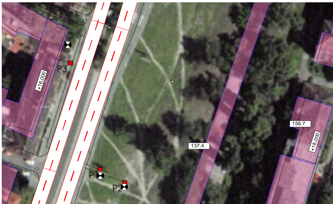
Figure 3: Measurement positions with parallel registration of hourly Leq levels
