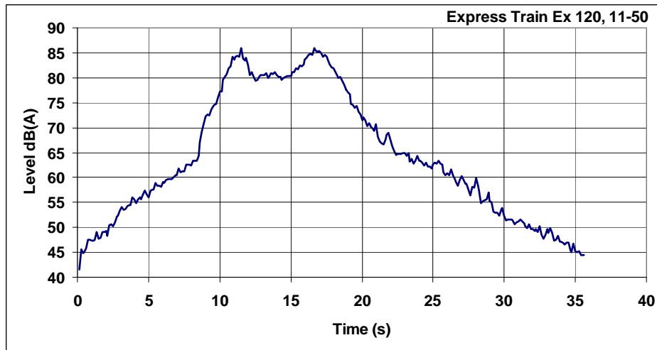
Figure 7: Measured LAF levels – Leq = 76,6 dB(A) with T = 35,6 s (1618 trains/16h)
