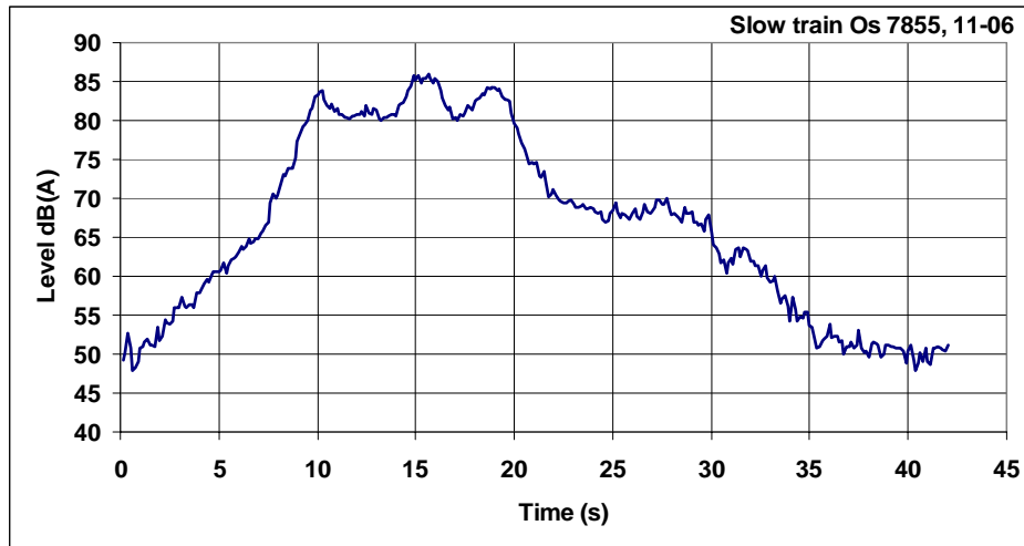
Figure 9: Measured LAF levels – Leq = 77,1 dB(A) with T = 42 s
