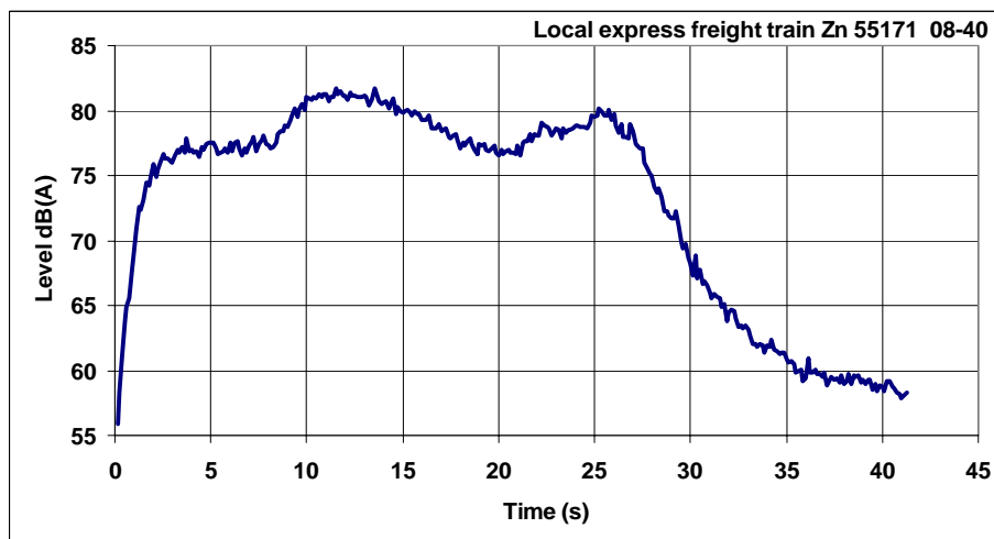
Figure 25: Measured LAF levels – Leq = 76,9 \text{ dB(A)} with T = 41,3 \text{ s} 1395 trains/16h – 46024 carriages/16h
