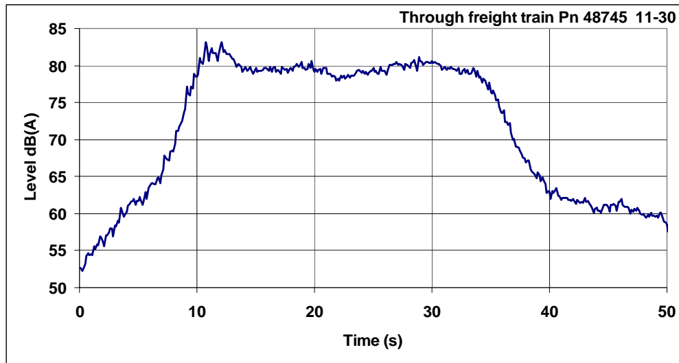
Figure 29: Measured LAF levels – L_{eq} = 76,9 dB(A) with T = 51,8 s 1112 trains/16h – 35583 carriages/16h
