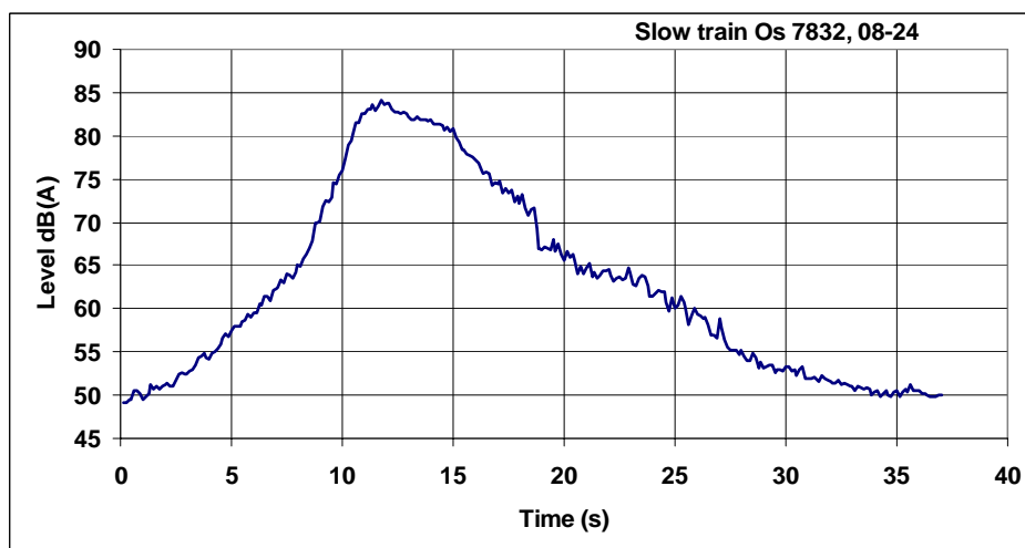
Figure 12: Measured LAF levels – Leq = 74,4 dB(A) with T = 37 s
